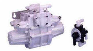
The Brix pump is a proportioning device, which pumps two liquids (e.g. water and concentrate) in an exact ratio. The particular ratio is determined by the pump design, and is thereby maintained precisely, independent of system flow or pressure changes, with no need to regularly readjust brix at the dispensing valve.
