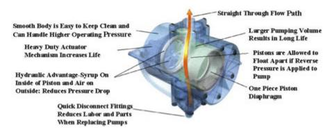
The above design configuration results in the greatest efficiency and lowest pressure drop every time the dispensing valve open and closes and thus insuring consistent beverage quality.
