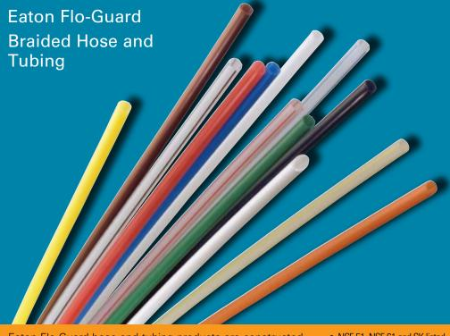
Eaton Flo-Guard hose and tubing products are constructed with a natural barrier inner core bonded to a modified copolymer cover. This combination allows for flavor protection and allows for reuse after cleaning. This barrier combination also allows for maximum flexibility, kink resistance and ease of installation in confined areas. It can also be permanently thermoformed in order to increase routing efficiency and reduce fitting usage.
