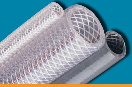
Eaton's line of PVC hose and tubing products are manufactured with materials which comply with FDA Regulation 21 CFR 177.1520 and are NSF-51 listed. These products are non-toxic and RoHS compliant. They are manufactured with a spiraled polyester yarn reinforcement and are longitudinally reinforced with a tracer yarn to reduce elongation under pressure. Applications include air lines, water lines, food and beverage dispensing, potable water transfer and pneumatic applications.
