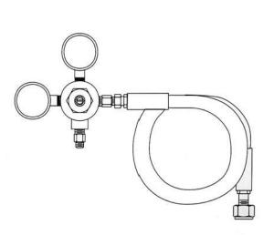
High Pressure Hose Assemblies are available for Wall Mount configurations in 3 ft (.91m), 6 ft (1.82m) and 9 ft (2.74m) lengths
