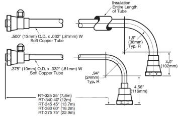
GRC Remote Condenser Line Kit Connections
