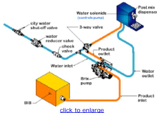
The Brix pump is designed with a vacuum shut off. The vacuum shut-off will automatically stop operation of the brix pump, when the concentrate BIB container is completely evacuated, by closing off the water inlet. When a new BIB is installed, the pump will automatically resume operation without the need to prime the system.
