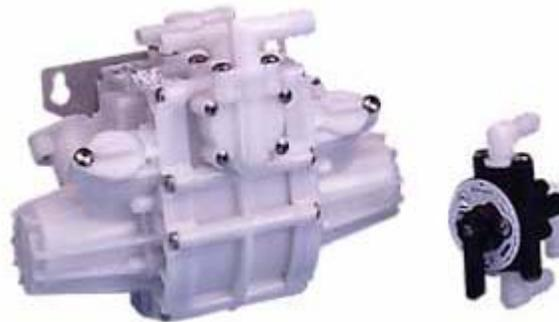
The Brix pump is a proportioning device, which pumps two liquids (e.g. water and concentrate) in an exact ratio. The particular ratio is determined by the pump design, and is thereby maintained precisely, independent of system flow or pressure changes, with no need to regularly readjust brix at the dispensing valve.
