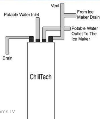
ChillTech Pre-Chill Technology effectively manages to pre-chill incoming water by using the purged water from the ice maker.
