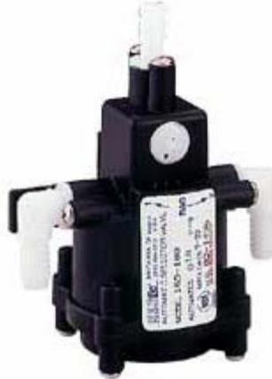
Eliminate the chore of replacing BIBs during peak business times. [An ASV](#) permits multiple ASV to be connected to a particular pump. Once the BIB on one side has completely emptied, the ASV automatically switches to the full BIB. An ASV provides uninterrupted drink dispensing and allows replacement of empty BIBs during off-peak hours.
