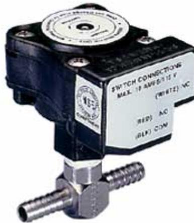
The [SOS](#) prevents the dispensing of carbonated water without syrup by stopping water flow at the dispenser valve - a particularly useful feature for lemon-lime (clear) sodas and drive-through windows. The SOS senses the pressure drop in the syrup line caused by an empty BIB and shuts off power to the valve's electric solenoid. The SOS automatically resets with the installation of a full BIB.
