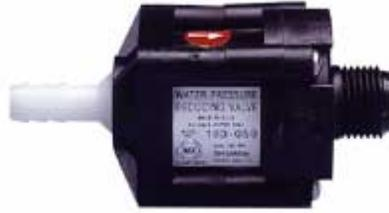
SHURflo's 183 series is a fixed water pressure reducing valve (non-adjustable). Its function is to minimize input water pressure fluctuations while guarding against high incoming spikes of pressure.
