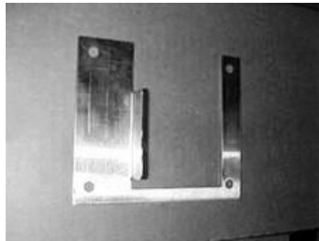
Figure 16. Ice Diverter for ED/DF models
